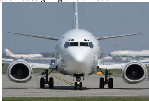
Figure 3. Front view of Boeing 737NG, flat engine bottom
