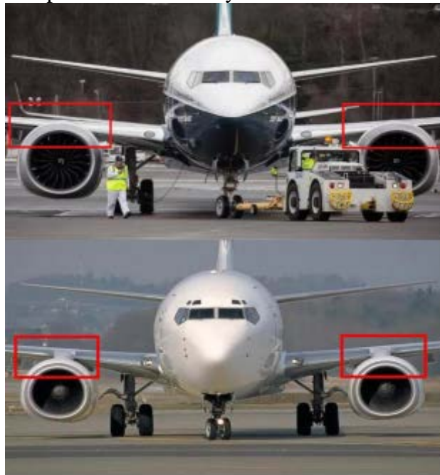
Figure 4. The figure above is 737MAX and the figure below is 737NG. The difference in engine position and is clear.
