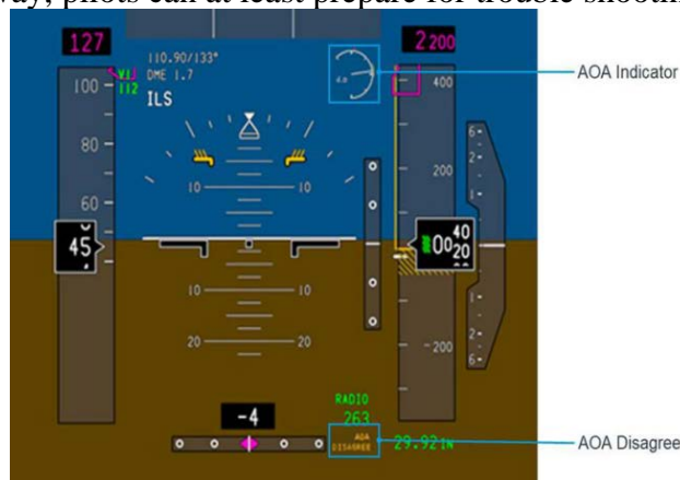
Figure 7. Angle of attack indicator and angle of attack disagree alert on the Primary Flight Display (PFD)
